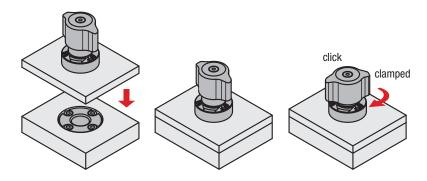
Ensure that the twist knob is in the "OFF" position. Set the ball lock pin in the premounted clamping plate. Turn the twist knob to the "ON" position. When fully clamped, an audible click will be heard.
