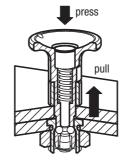
To remove, press the knob down and pull the ball lock pin out of the bush.
